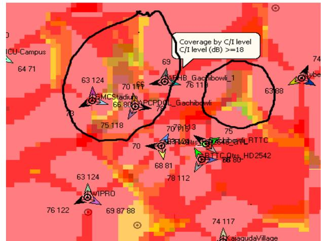
Fig. 6. Interference zones occurred in manual planning
