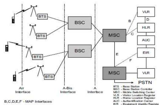
Fig .1. Outline of GSM network architecture
